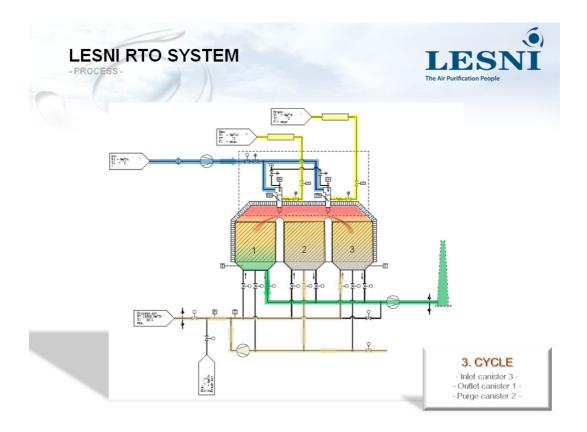
The LESNI Regenerative Thermal Oxidiser; type REF has a bypass function, where the unclean air is lead directly to stack, bypassing the hot oxidiser for safety and maintenance.
