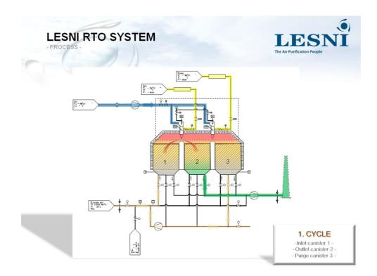
The same principle of operation is then used in rotating sequence of chambers / canisters for cycle 2 and cycle 3 (see picture cycle 2 and cycle3).
